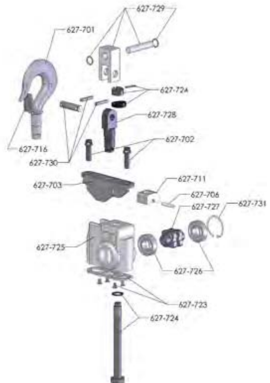
TRIPLE REEVED SUSPENSION & SHEAVE HANGER
